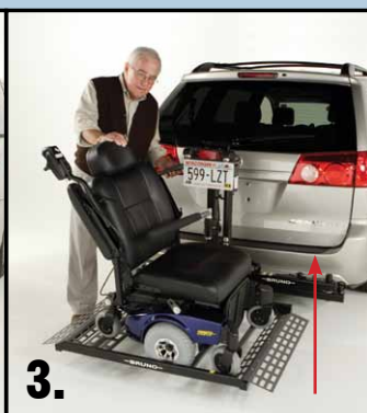
3. Raise lift to automatically secure powerchair.
