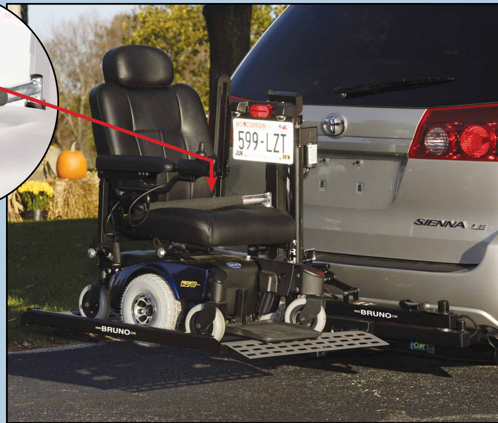
Automatic Hold-Tite for Powerchairs (HTP) Version
