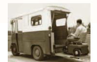
Ralph equips an old Post Office Jeep with a custom-built hydraulic tailgate lift along with homemade hand controls.
